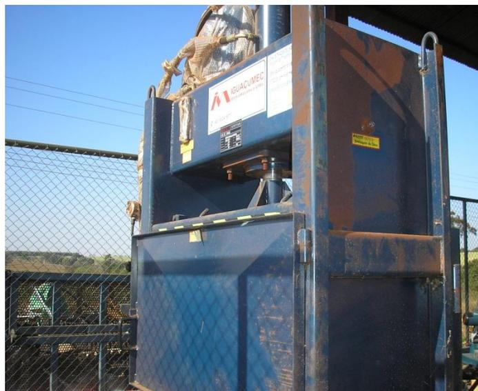
**FIGURA 35 - PRENSA HIDRÁULICA VERTICAL**
